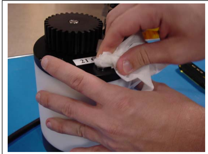
Figure 4-7: Cleaning Excess Oil from Fill Plug
