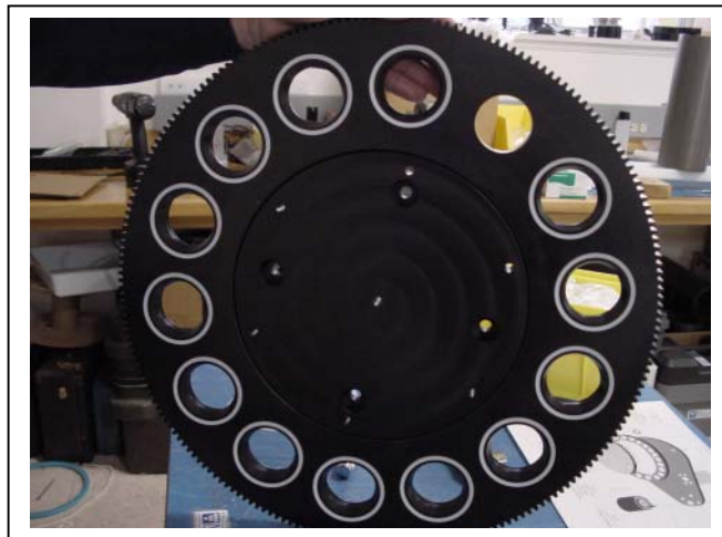
Figure C-5: Variseals® in Gear Ring Grooves
