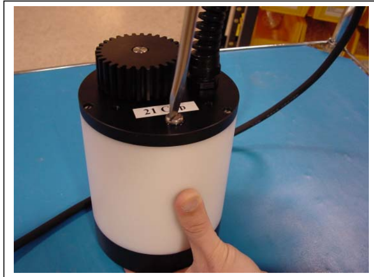
Figure 4-5: Back Off Fill Hole Screw and Press Up on Bladder
